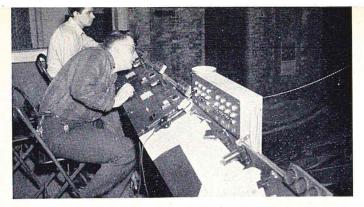
Control panels for the engineers and dispatcher. The board in the foreground is for the dispatcher. Bob and another engineer operate trains from the control panels in the balcony. Each engineer is provided with signal lights, a switch to make the train move in either direction, a rheostat for controllng the speed of the train, a time table, and an ampere indicator. The balcony is reached by climbing the regulation 19-inch railroad ladder.
